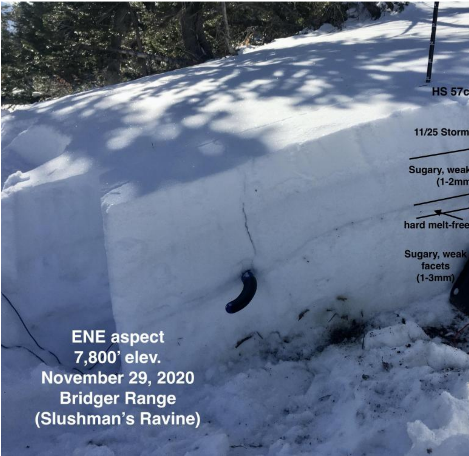
This snowpit at Bridger Bowl was on a shaded ENE aspect at 7,800'. The lower two thirds are mostly sugary, weak facets with a hard crust in the middle. This weak snow is not the best foundation for the winter's snowpack. Photo: GNFAC
