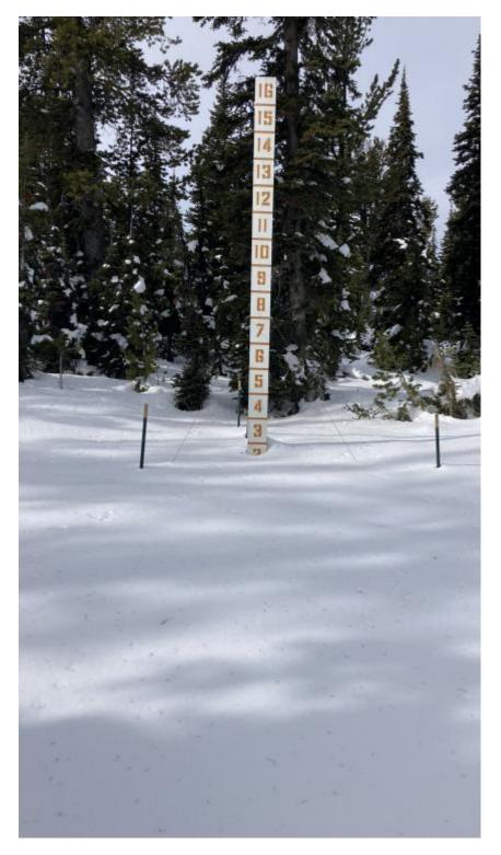
Went to do maintenance on the Sawtelle Snowfall weather station at 8800 ft just off the Sawtelle Mountain Road. Continuous snowcover starts around 8000 ft. At 8800 ft there is ~20" of snow with a mix of hard crusts and weak facets. These weak layers near the ground will be something to watch once snows again. Photo: GNFAC
