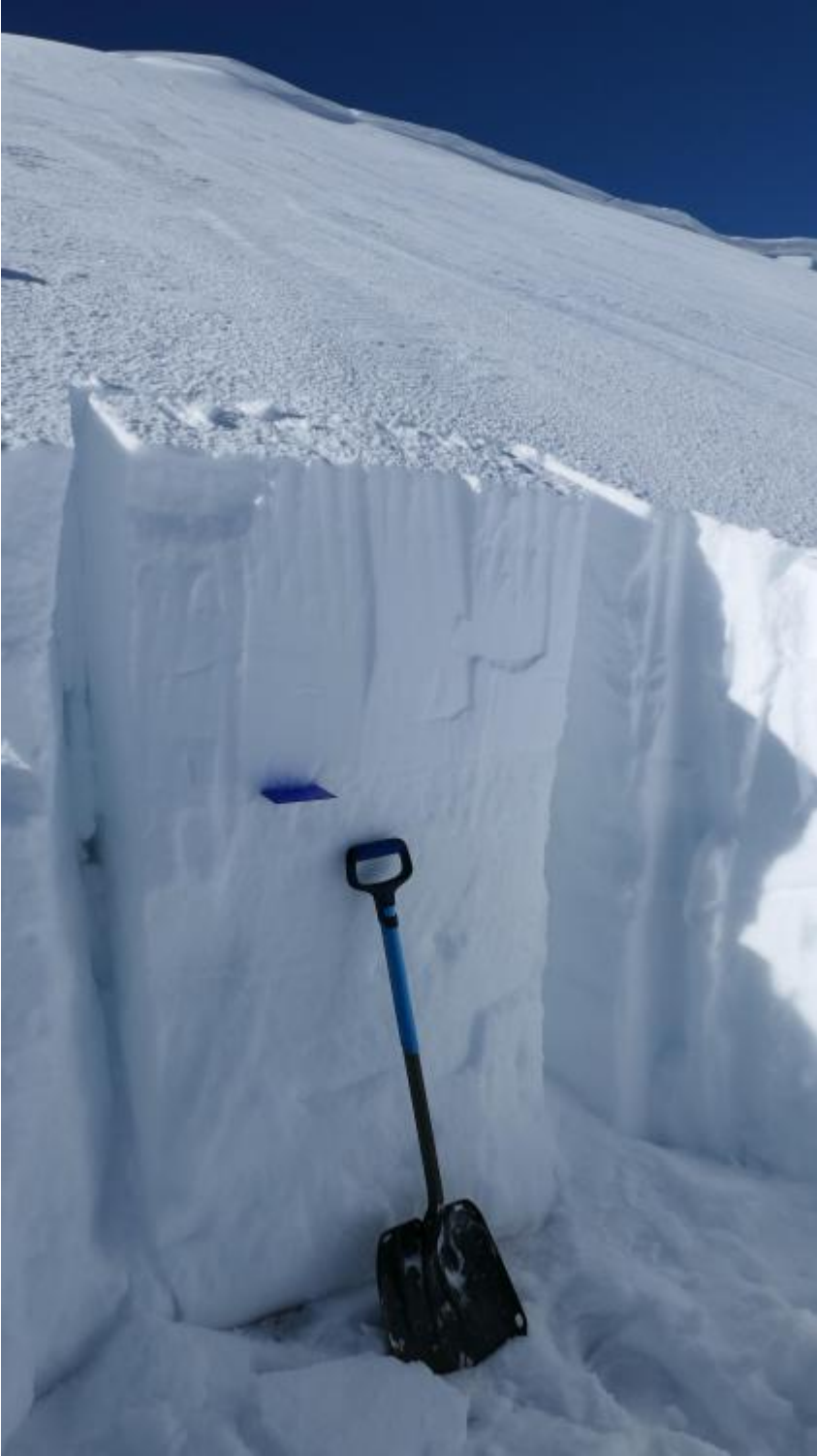
A snowpit in the flank of an avalanche on Henderson Ridge. The blue crystal card marks the interface between the slab and the weak layer. Photo: GNFAC
