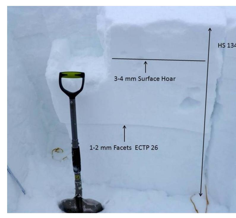
A layer of facets buried mid pack is the layer of concern. Although it's taking hard force to get this layer to fail, it continues to propagate in stability tests. This layer should be assessed before committing to avalanche terrain. Photo GNFAC
