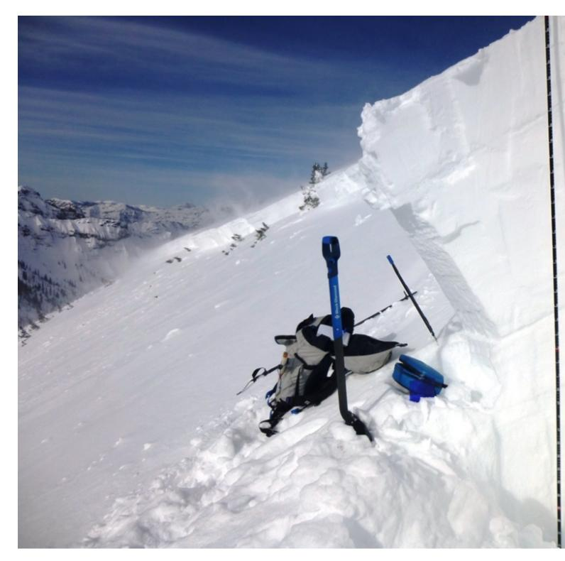
The crown was 3-4 feet deep. The avalance was triggered approximately 50 feet below the crown on a rock band. Facets that formed in the early season fractured and propagated across the slope. Photo: GNFAC
