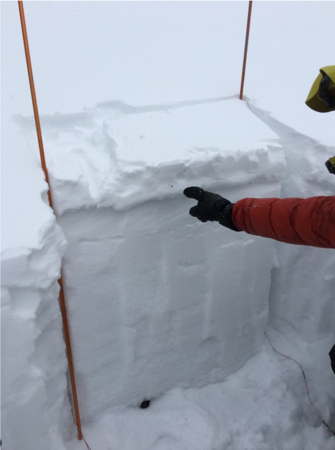
A 2" thick wind slab is cracking, whumphing and breaking easily in stability tests (ECTP3). This was seen in the Throne area of the northern Bridgers. Skiing and sledding was reported to be "awful" from the winds. Photo: B. Nobel
